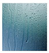
External condensation (dew) can occasionally occur on highly insulating glass units in temperate climates. Such occurrences will only happen on cloud-free nights when there is little or no wind and usually when a warm front follows a dry spell
